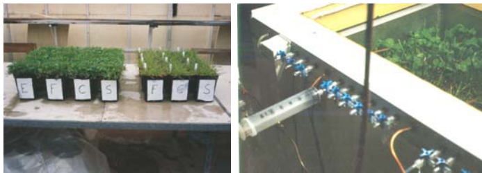
Figure WP1.2a Pots with grass-clover for ^{15}\text{N}_2 -labelling and close up of growth cabinet. Water is provided through a silicon tube to each pot connected to a valve on the outside.
